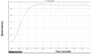
Fig.16 Simulation result of bidirectional full bridge DC-DC converter with flyback snubber with DC Motor – Boost closed loop operation [Speed curve] with a speed of 58.1rad/sec
