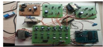
Fig.23 Photograph of prototype converter
